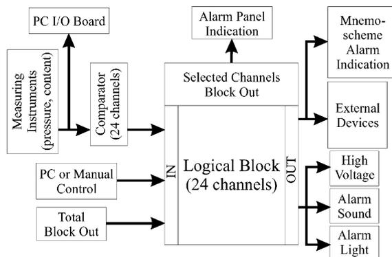
Fig. 4. Block diagram of alarm/interlock subsystem.
