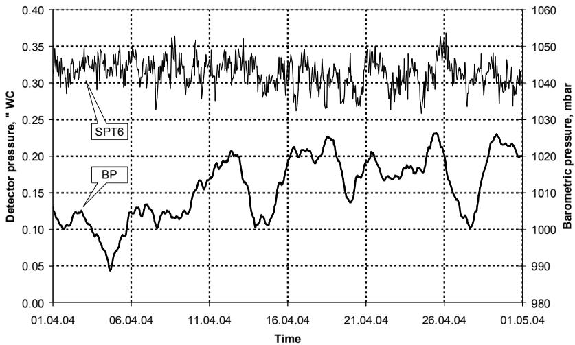
Fig. 2. South MuTr output manifold and barometric pressures chart.
