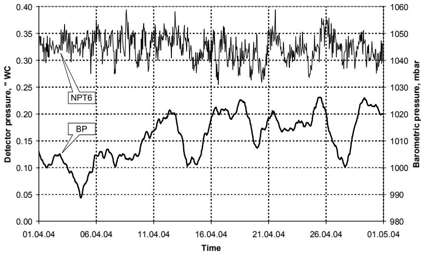
Fig. 3. North MuTr output manifold and barometric pressures chart.
