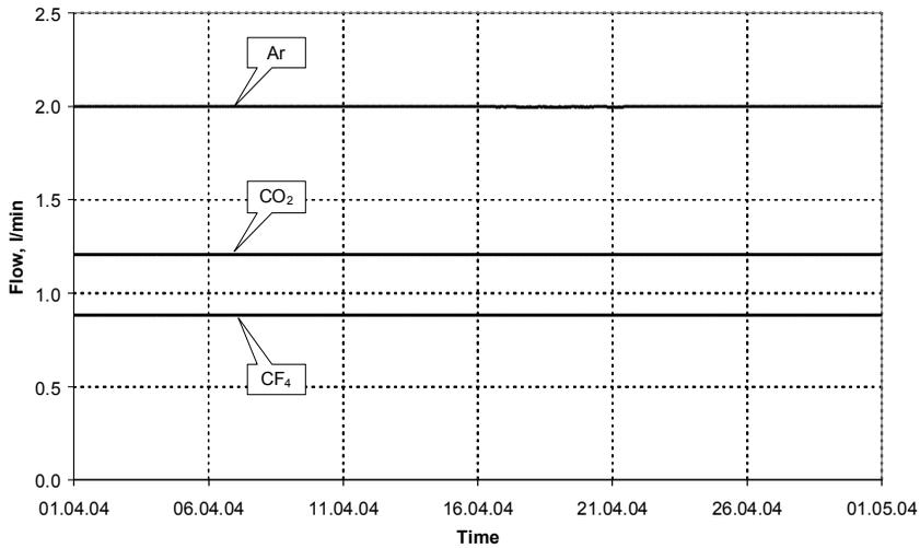
Fig. 4. Ar, CO<sub>2</sub> and CF<sub>4</sub> flows.
