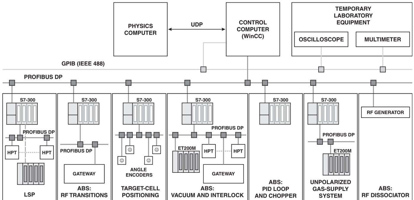
Fig. 7. Structure of the control system for the polarized internal target (PIT) of ANKE-COSY. The unpolarized gas-supply system is a temporary diagnostic tool, described elsewhere [13].
