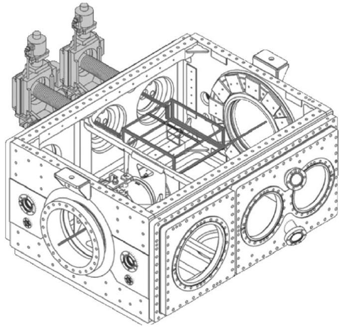
Fig. 4. 3D CAD drawing of the ANKE-target chamber with the two manipulators carrying the frame with a diaphragm used for beam diagnostics. The COSY beam enters the chamber from the left.
