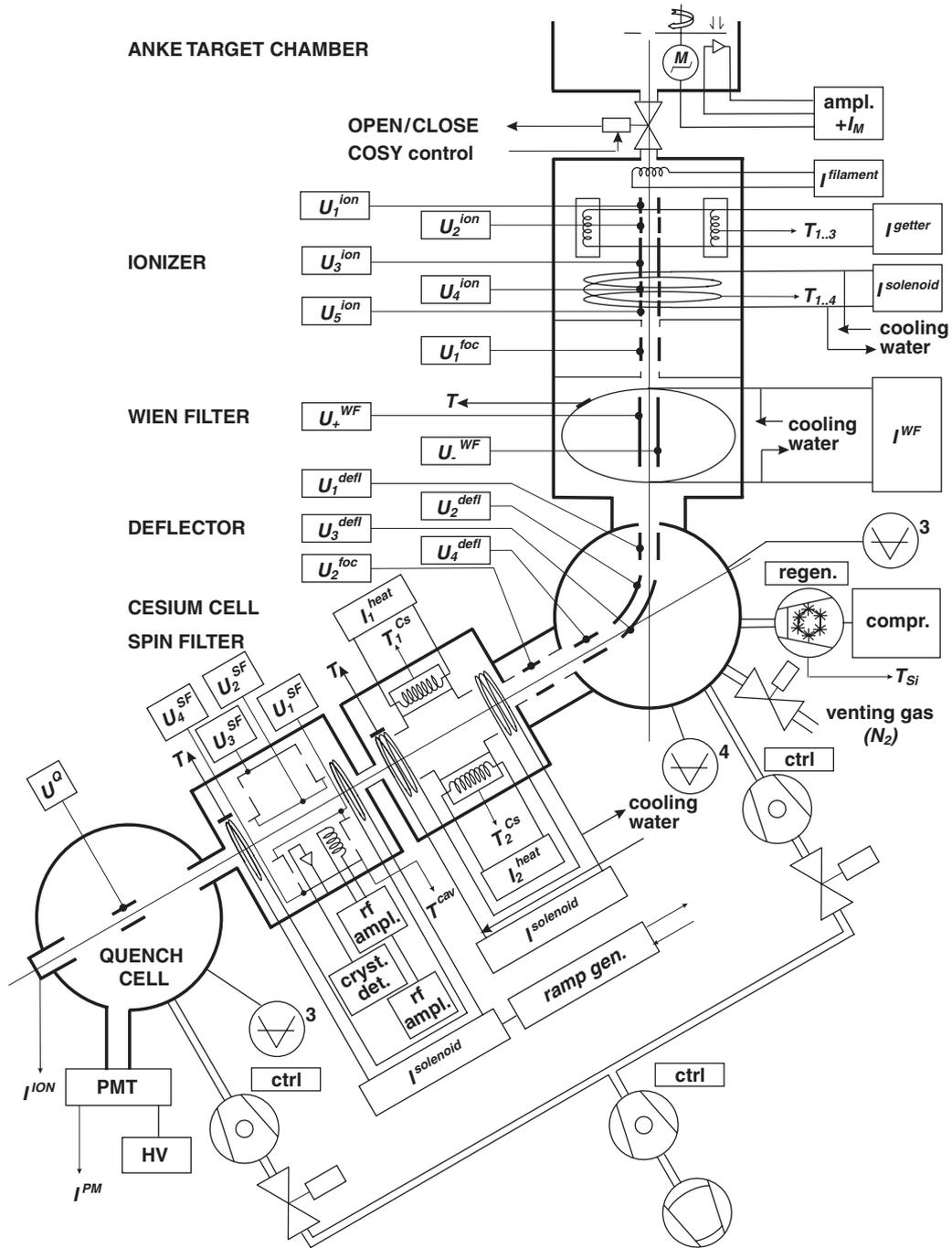
Fig. 3. Scheme of the controlled components of the Lamb-shift polarimeter with beam chopper in the ANKE target chamber, ionizer, Wien filter, 60° deflector, cesium charge-exchange cell, spin filter, and quench chamber. The symbols are explained in the caption of Fig. 2.
