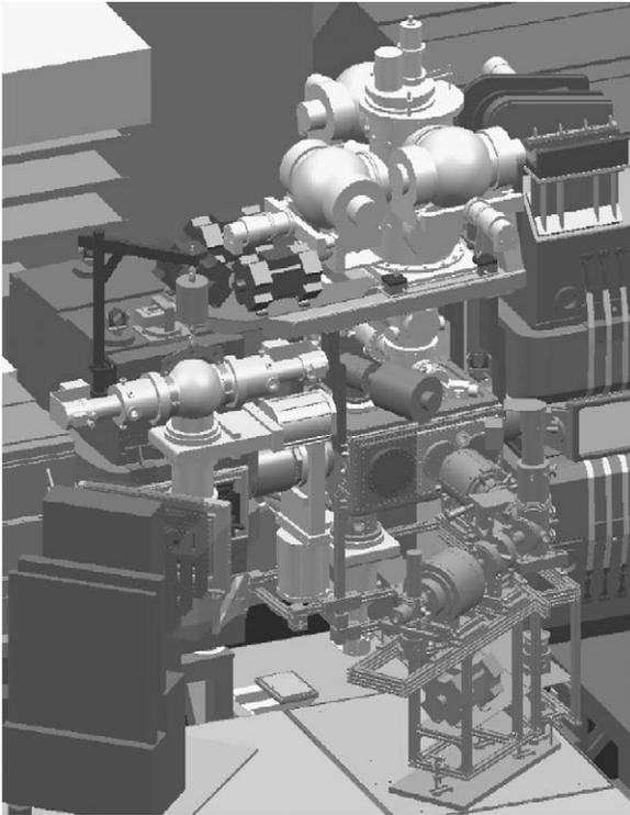
Fig. 1. 3D CAD drawing of the polarized atomic beam source (vertical) and the Lamb-shift polarimeter (horizontal, with the 60° deflector) at the ANKE-target chamber in front of the central spectrometer dipole magnet (right-hand side).
